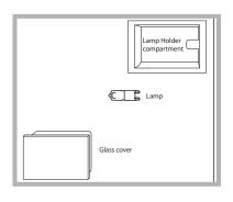
2. Remove the light bulb and replace it with a similar one: halogen lamp voltage 230 V, wattage 25 W, cap G 9.
